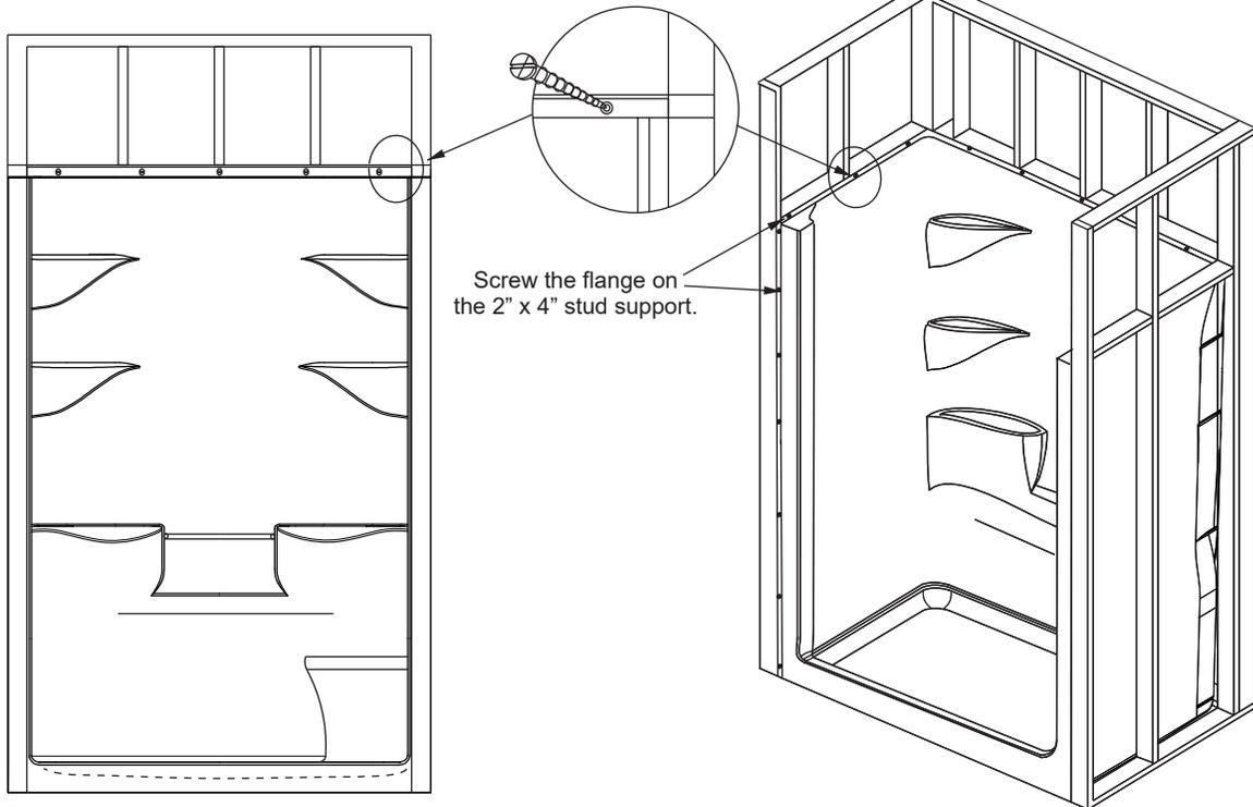
FIGURE 3 - MELROSE FASTENING WITH DRYWALL SCREWS
