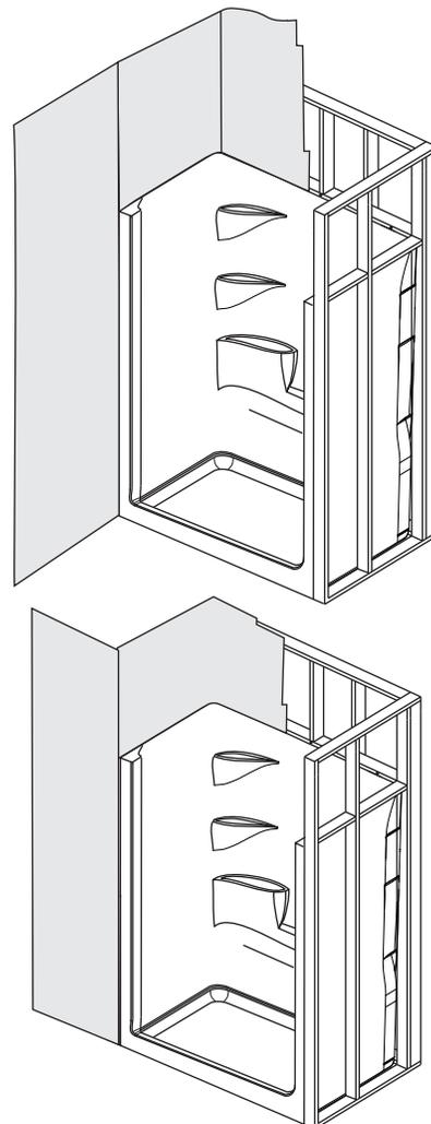
FIGURE 5 - THE INSTALLATION OF A STUD IS MANDATORY FOR ADEQUATE BEARING SURFACE TO SCREW THE DRYWALL TOO.
